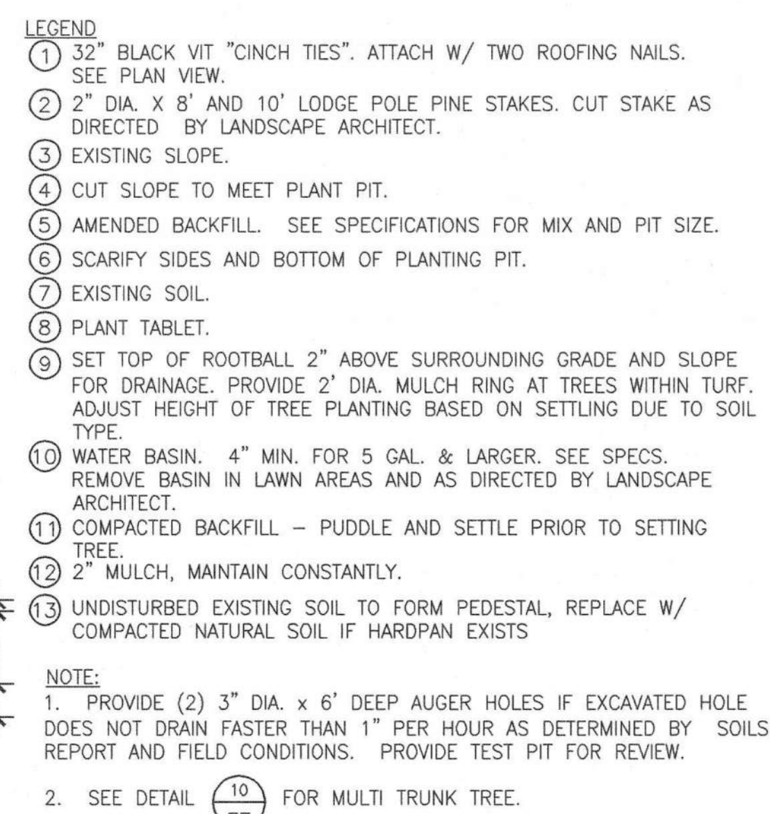
TREE STAKING AND PLANTING ON SLOPE 1/4" = 1'-0" DT02LP12 20
